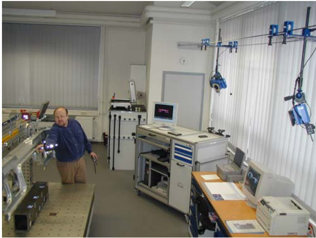
Fig 1: In the V-STARS measuring cell, where the tactile portion of the component measuring processes is performed, the INCA3 cameras are suspended in mid-air.
