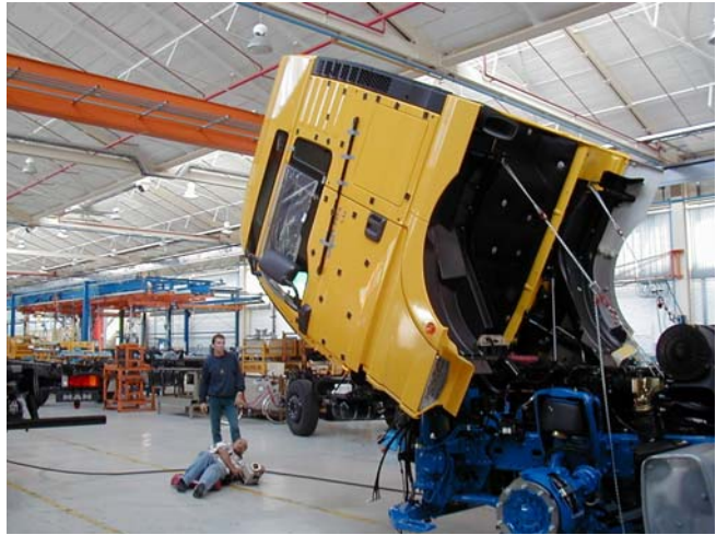
Fig 2: Photogrammetric measuring of deformation in cabs directly during manufacturing.
